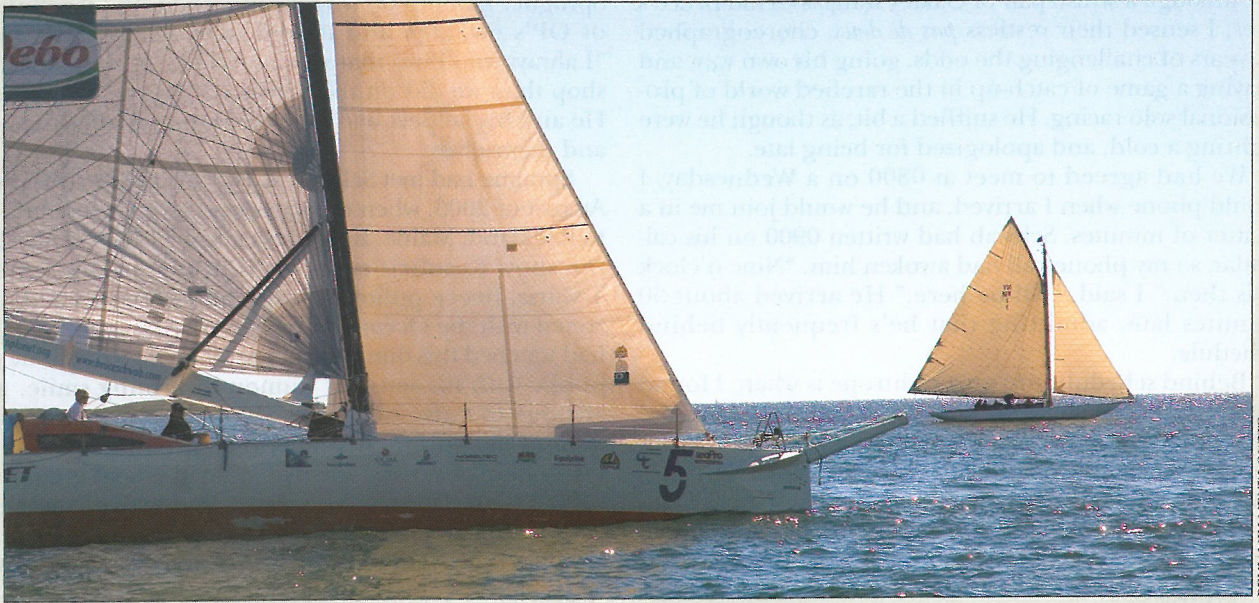
What a difference a rule makes. In light air, OCEAN PLANET (plumb ends, long waterline) sails off Boothbay Harbor, Maine, in company with the restored New York 30 ALERA (long overhangs, short waterline): different times, different rating rules.
