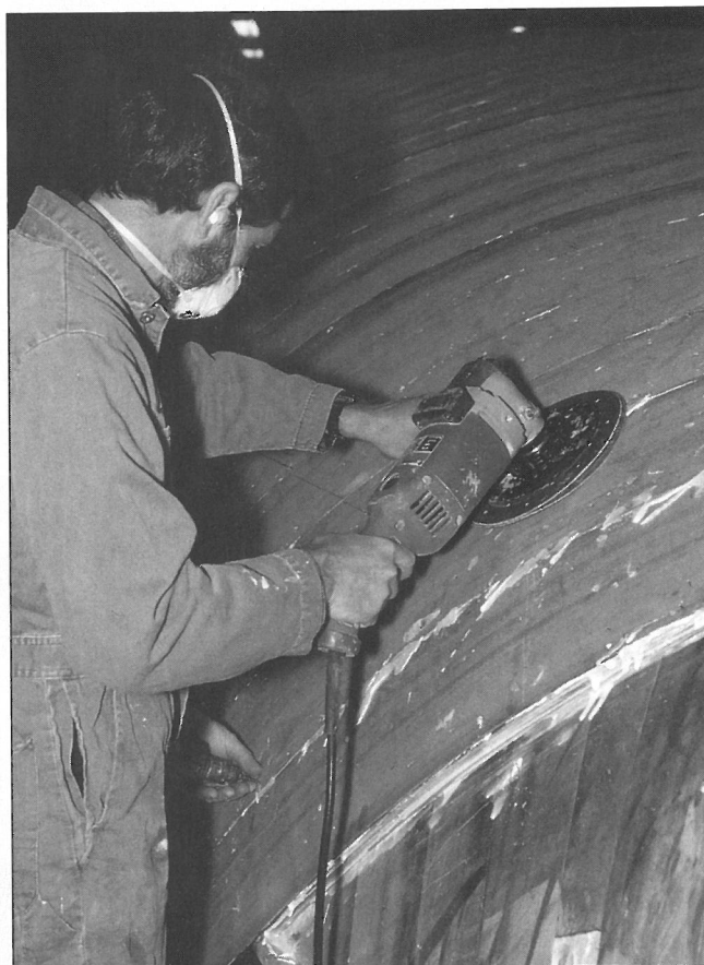
As Steve Rander sands off the excess epoxy on the first of the exterior diagonal veneers, a co-worker (see hand, bottom left) removes the temporary fastenings.
