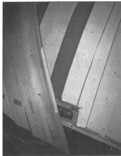
A 1" layer of Klegecell—a closed-cell PVC foam core—acts as a vertical web separating the two skins of wood veneers and 'glass cloth, and creating a stiff, light structure.
